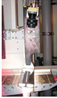
**Figure 5:** Camera-based inspection system.
